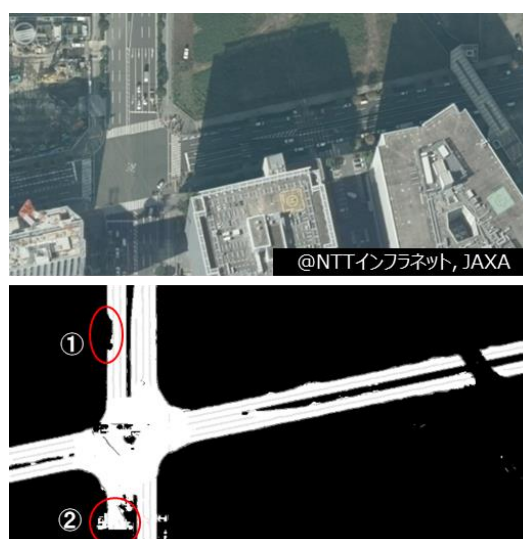
Fig. 2 inference result, two circled area shows the examples of miss-extraction
