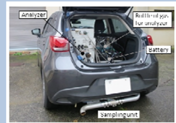
Figure 5-1 PEMS setup for test vehicle
