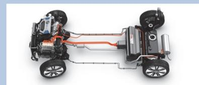
Figure 1-6 twin up!の駆動系のレイアウト
