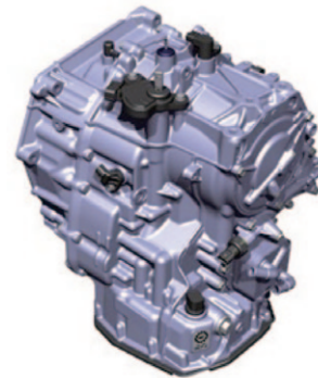
Fig. 5 External View of Honda N-Van CVT Unit
