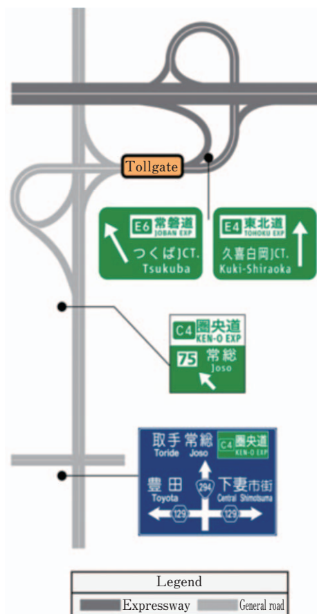
Fig. 3 Example of signs at expressway entrances (1)
