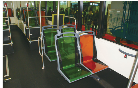
Fig. 11 Plastic seats proposed for urban buses.
